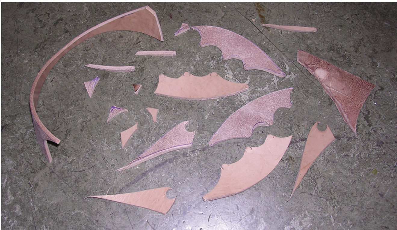
Fig. 6: Total scrap from one pair of Ramshaw boots (photo F. Himmler)
