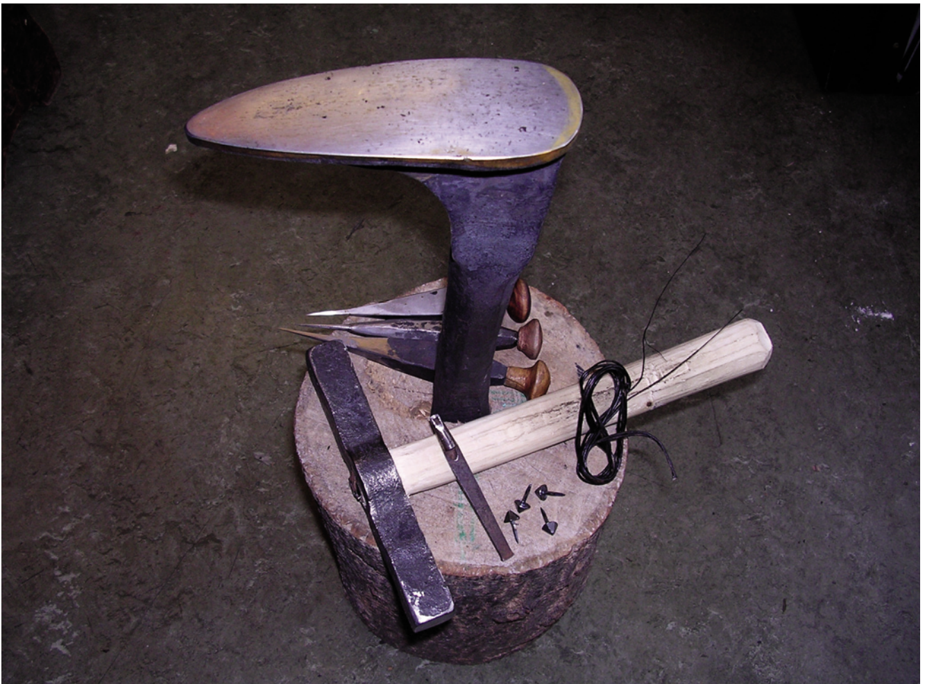
Fig. 1: Replicas of Roman tools: nailing anvil after the Saalburg example, awls after the finds from Vitudurum, shoemaker's hammer after the example from Lousanna-Vidy. (Photo F. Himmler, replicas made by J.-M. Coronat, Musée du Fer, Vallorbe CH)
