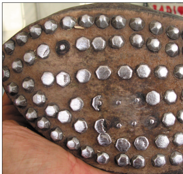
Fig. 14 (left): only the shafts remain of 6 totally worn down hobnails. Several others will soon follow.
