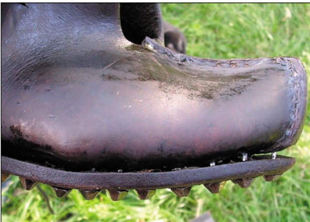
Fig. 15 (right): the nails come loose and so does the sole.
