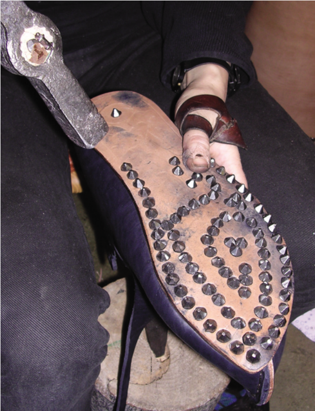
Fig. 8: Nailing the sole. (Photo F. Himmler)
